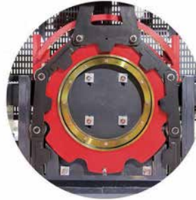
Chain-Tooth Slave Mechanism (Upper Rotation)
