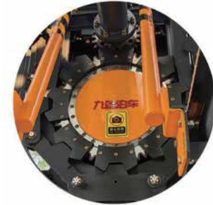
Chain-Tooth Drive Mechanism (Lower Rotation)
